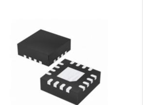
Part Number: SI53322-B-GM Manufacturer Energy Micro (Silicon Labs) **Description** IC BUFFER 1:2 LVPECL 16QFN Data sheet: Si53320-28
